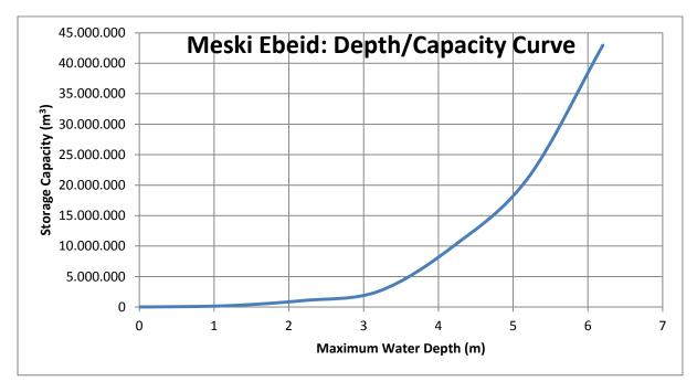
The above curve is based using the digital elevation data extracted from Google Earth. A topographical survey done on the ground using say a Total Station would provide a more accurate relationship between depth and storage capacity.
