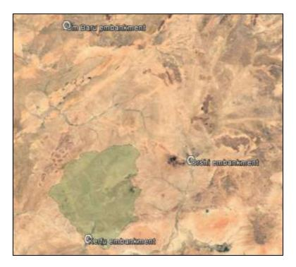
The catchment area of Kerfu dam is about 113km<sup>2</sup>. This is considerably less than the catchment of Orshi embankment dam which is over 300km<sup>2</sup>.
